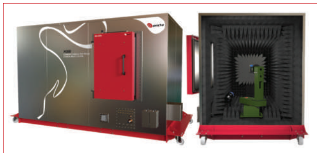
▲ Fig. 3 H300 CATR+DFF+SNF 5G OTA Test System by EMITE.
