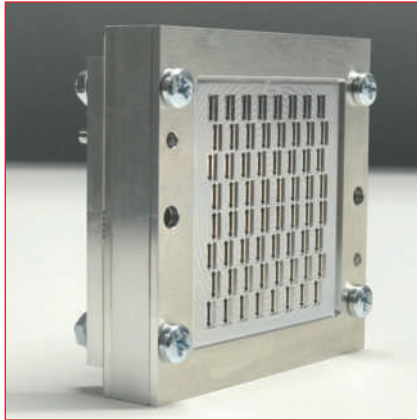
▲ Fig. 7 The single polarization Gapwaves antenna is an 8 x 8 slot array configured as 4-slot subarrays in eight columns and two rows.
